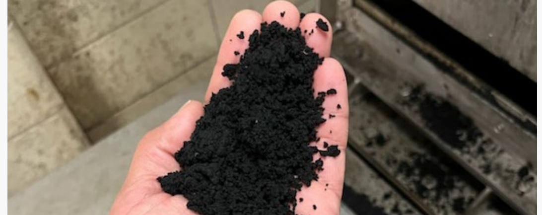
Dewatered biosolids product
